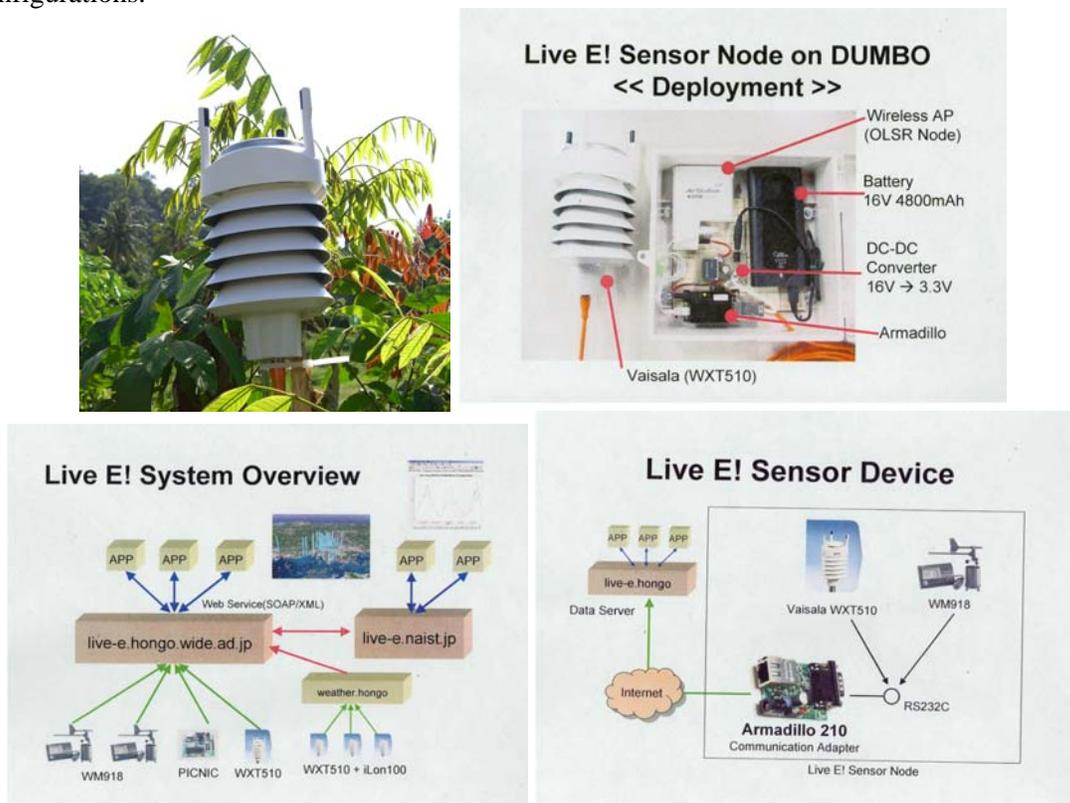
Figure 3: Sensor equipment deployed in DUMBONET and its connectivity configurations
